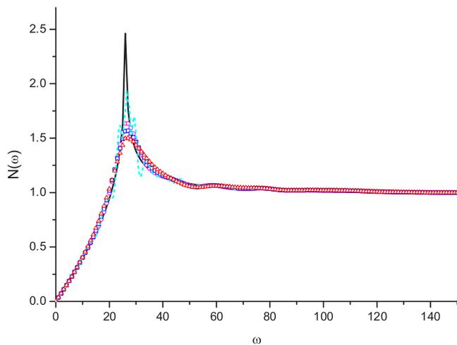
FIG. 4. Extracted DOSs at  $T = 150$  K with  $\alpha = 1$  (dashed line), 50 (red circles), 100 (blue squares), and 200 (magenta triangles). The solid line denotes the  $d$ -wave DOS [Eq. (10)] at  $T = 150$  K.
