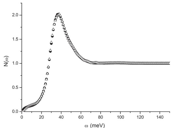
FIG. 5. Extracted DOSs from the  $I(V)$  curve measured at  $T = 4.2$  K with  $\alpha = 50$ ,  $\omega_0 = 30$  meV,  $s = 1$  (filled circles), and  $s = 2$  (open triangles).
